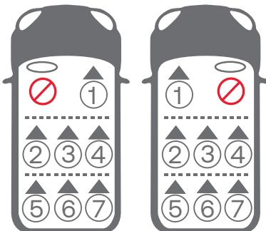
Before you purchase the vehicle, check that it is equipped with the appropriate anchorages.
